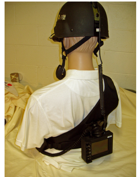
WalkAbout LCD mounted on the rear. WalkAbout base can be mounted on the chest plate to balance the weight making it more comfortable to wear.
