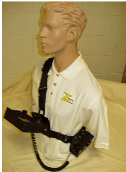
WalkAbout LCD mounted on chest plate with the WalkAbout base on Waist strap. WalkAbout base may be worn on the belt if desired.
